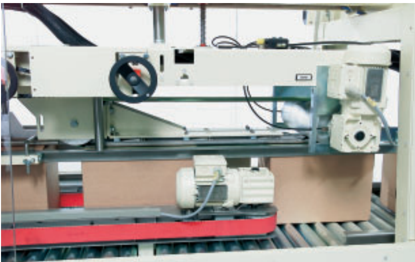
The front stop-end flaps and lateral flaps are automatically folded and glued (top picture).
